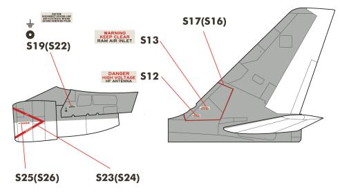
APPLY INTAKE MARKINGS ON BOTH SIDES OF THE NACELLES.
